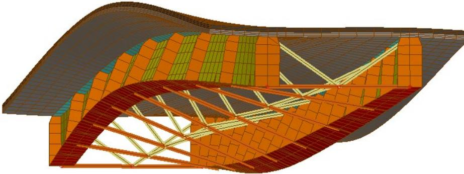
Figure 5: Deformed shapes for the single span case. Torsionless and horiz. braced
