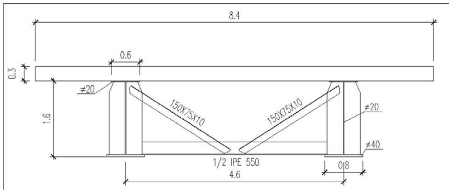
Figure 4: Section geometry used for the test cases
