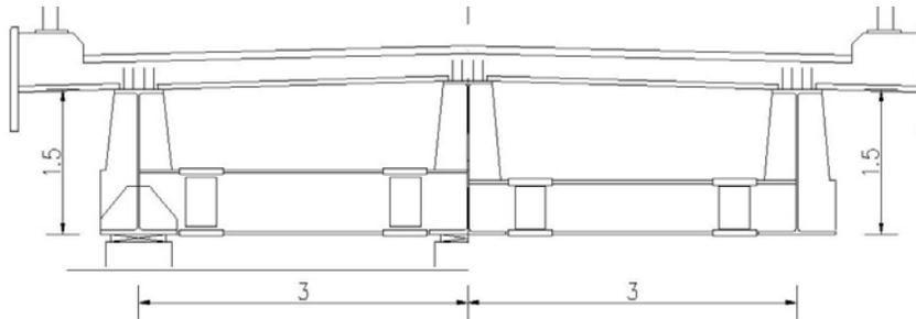
Figure 2: Typical cross section of the Asti-Cuneo motorway overpasses
